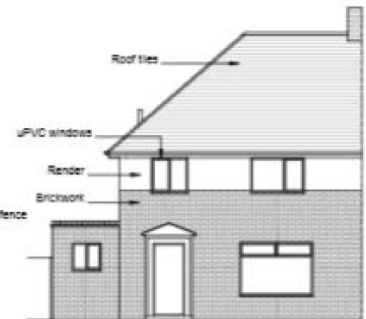
Existing Front Elevation 1:100
