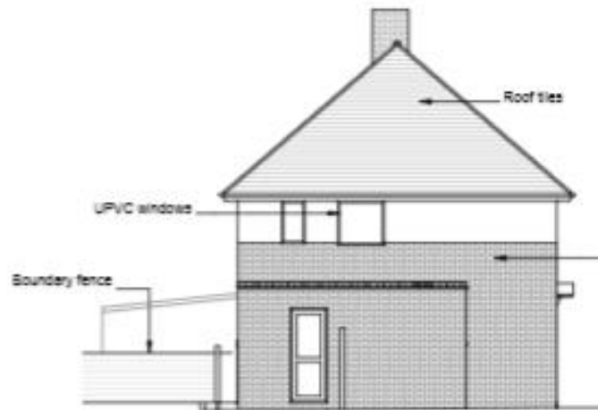
Existing Side Elevation 1:100
