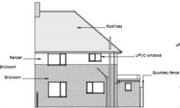
Existing Rear Elevation 1:100
